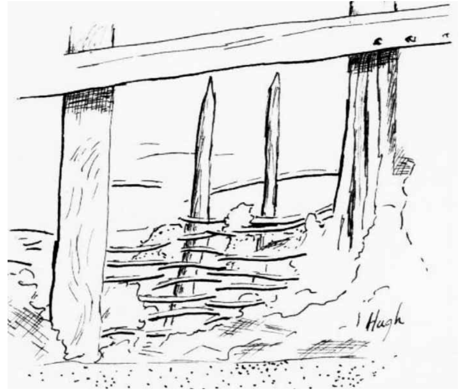
Wattle and daub revealed in a ruined wall.
