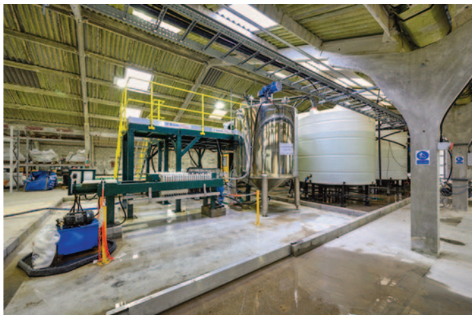
Inside British Lithium's pilot plant which produces lithium carbonate as a finished product. (Image: British Lithium)
