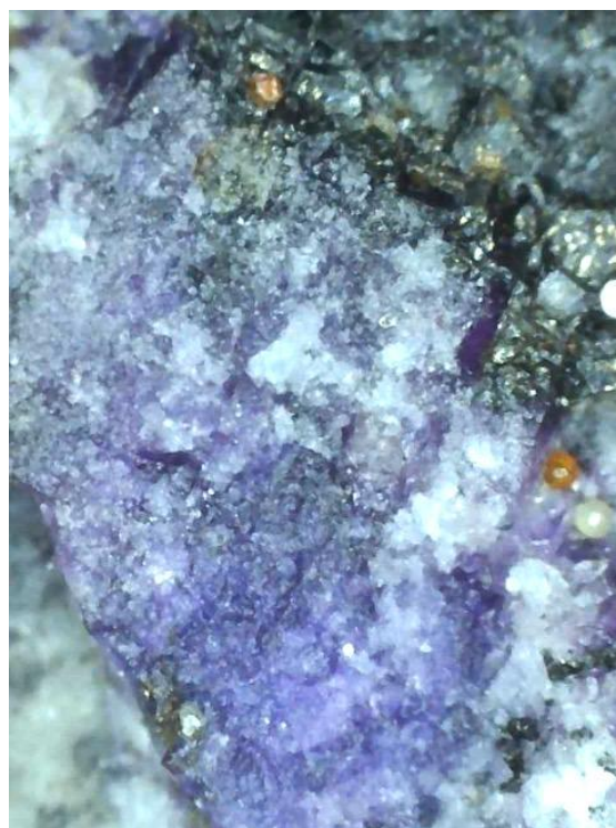
Traces of Blue John Fluorspar seen in the sample (*30 magnification)
