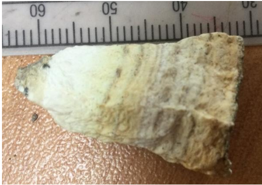
Sample of baryte from the talus piles. Baryte and calcite are the two most common gangue minerals left behind after the extraction of galena (lead ore).
