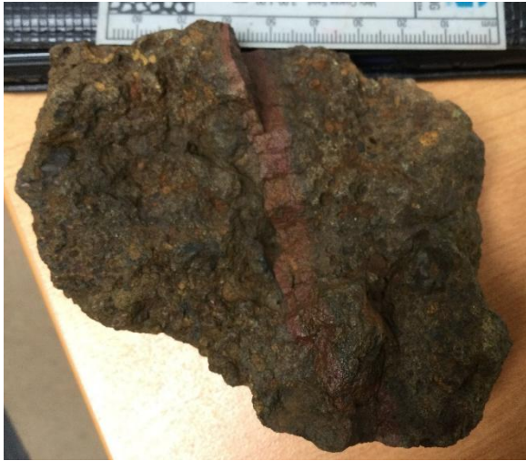
Sample from the basalt lava showing an iron concentrated vein and pieces of basalt fragments within the sample indication an aerial component (ash) to the deposit
